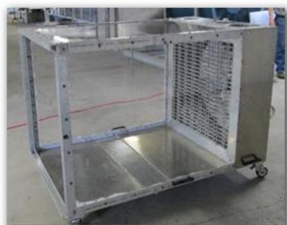
Figure 1. Miniature wind tunnel used to compare spray qualities for drift
