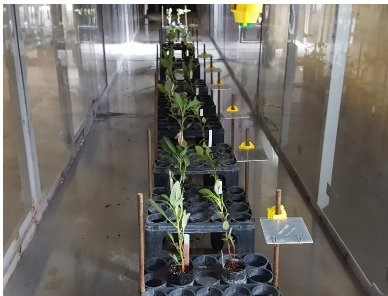
Figure 1. Herbicide drift study conducted in the low speed wind tunnel with waterhemp ( Amaranthus tuberculatus ), Palmer amaranth ( Amaranthus palmeri ), and drift collectors (Mylar cards) positioned at different downwind distances from the nozzle.
