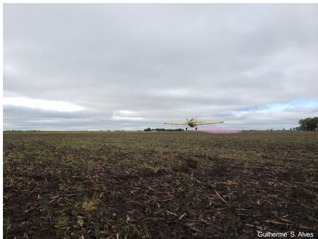
Figure 1. Air Tractor 802A aircraft used to spray glyphosate tank-mixed with a drift-reducing adjuvant in South Dakota.
